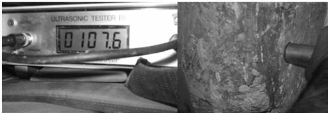
Figure 2: Process of Realization of the Ultrasonic Velocity Testing, Using a “Ultrasonic Tester”, in a Piece of Reinforced Concrete under Investigation
